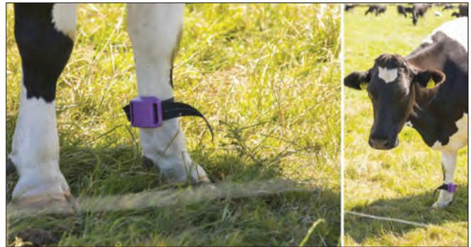
FIGURE 1. Cows with long-range pedometers (LRPs) attached on one of their front legs as part of our smart dairy farm setup.
